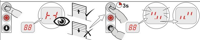
2. Move to OPEN final limit position and adjust S3 OPEN limit switch
